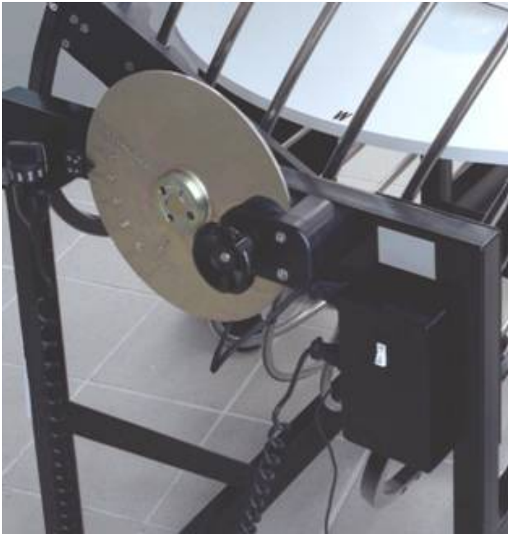
Fig. 5 ( Back ) View of the control end of the Model 126 Heliodon.
