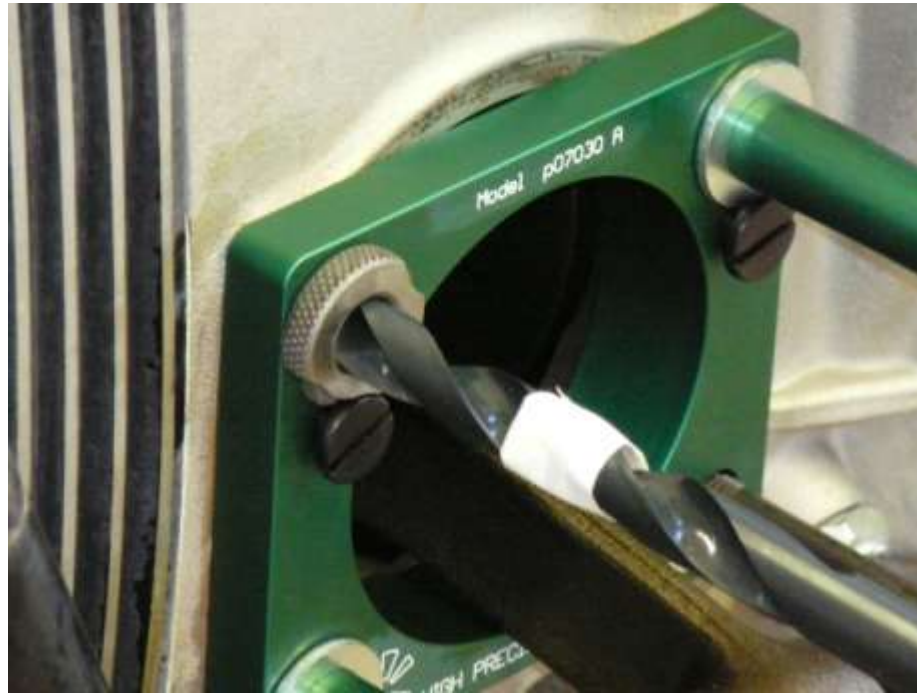
Figure 4: Drill pilot hole.
