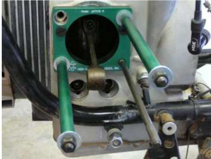
Figure 2: Proper HPD Stud Tool installation.
