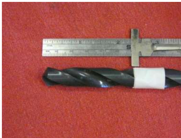
Figure 3: Place a tape marker on drill bit 58mm from tip.
