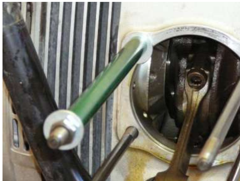
Figure 10: Installation of head stud.
