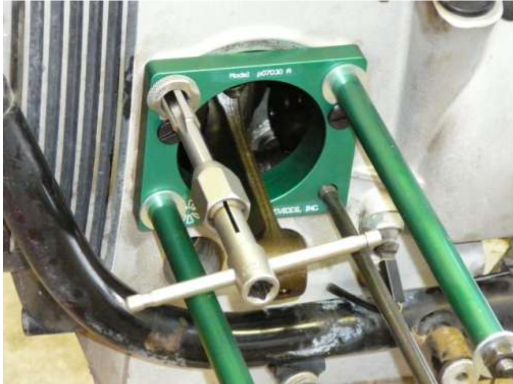
Figure 5: Tapping the hole.
