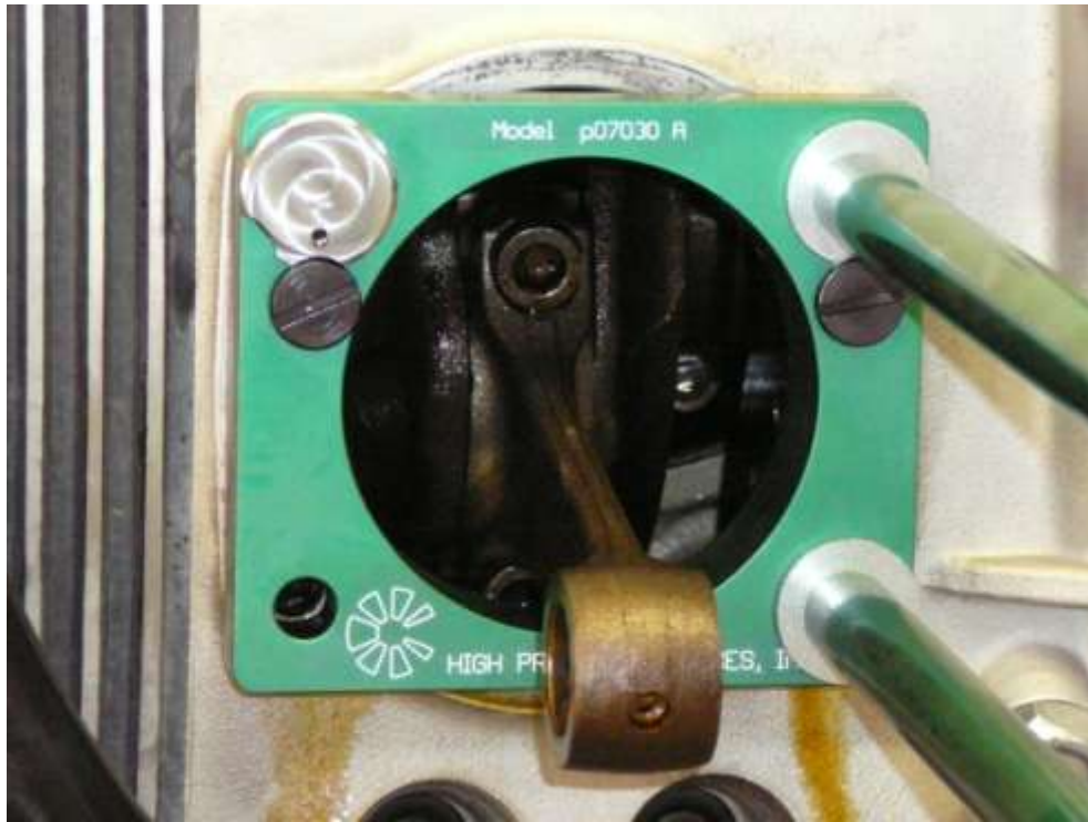
Figure 8: Mounting configuration for oil passage drilling.
