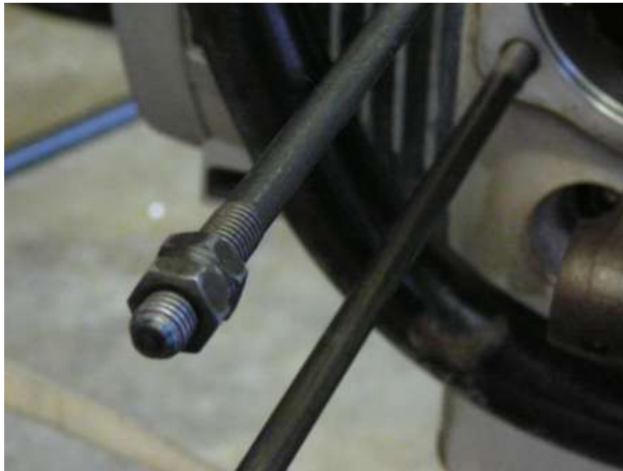
Figure 1: Removal of stripped stud.
