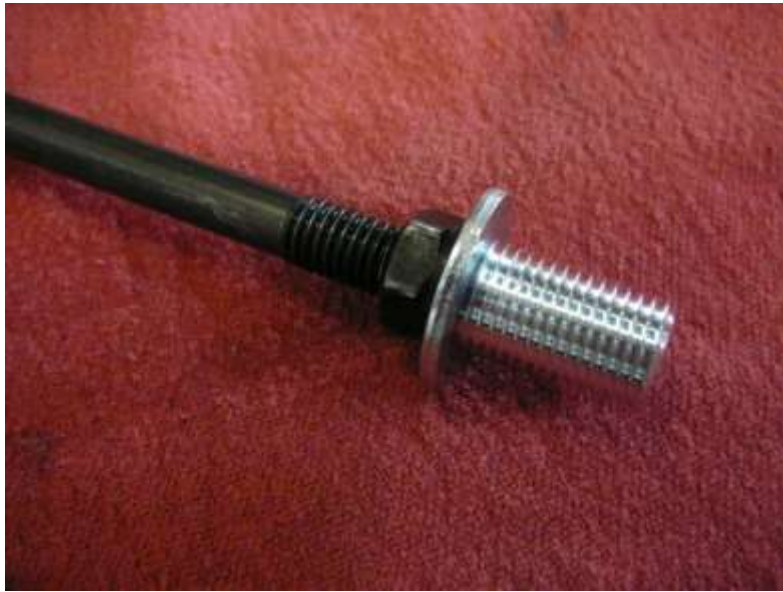
Figure 6: Installation setup for threaded insert.
